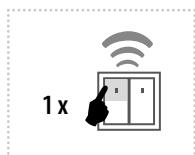
The output contact will be opened by pressing the button and closed after the set time interval has elapsed.
