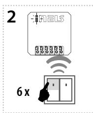
Assignment of the delayed on function is performed by six presses of the selected button on the RF transmitter (must be a lapse of 1s between individual presses).
