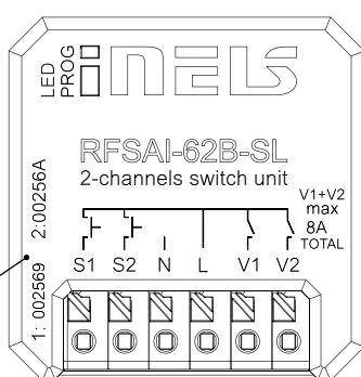
Addresses listed on the front side of the actuator are used for programming and controlling the actuator and individual RF channels by control units.
