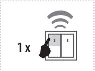
The output contact will be closed by pressing the button.
